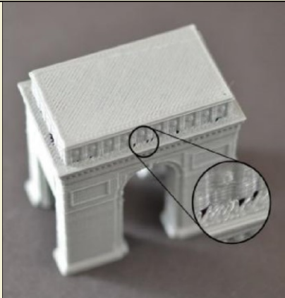
Gaps in Floor Corners
