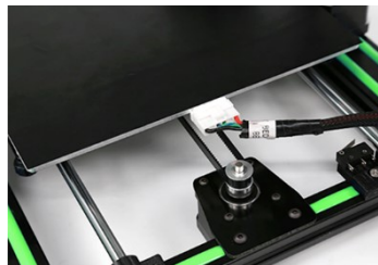
Hotbed Please insert the hot bed wire tightly in case of burning out.
