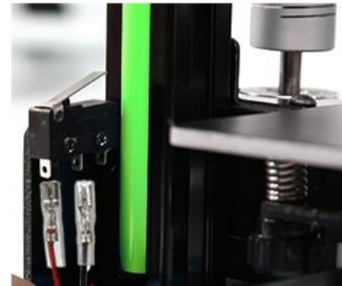
Z Axis Limit Switch
